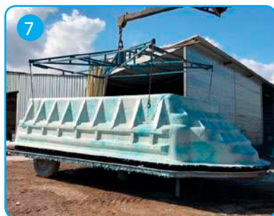
7 Desmoldeo Remove swimming pool
